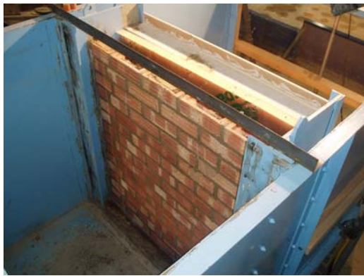
Figure 2 Testing arrangement for cavity wall (facing brick external face and Aircrete blocks on internal face) with rigid closed cell insulation
