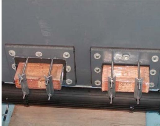
Figure 1 Testing arrangement for facing bricks
